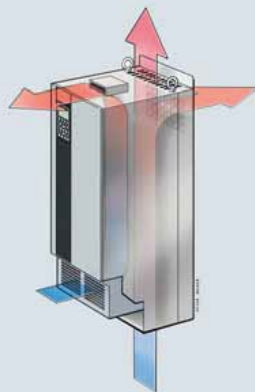
Minimal airflow over electronics Complete separation between back-channel cooling air and the internal electronics ensures efficient cooling.
